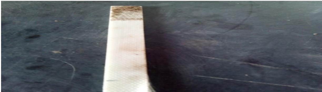
Fig.4 Tensile test specimen of dimensions 250x25.4x4mm.
