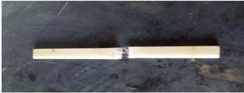
Fig.7 bending test specimen after test
